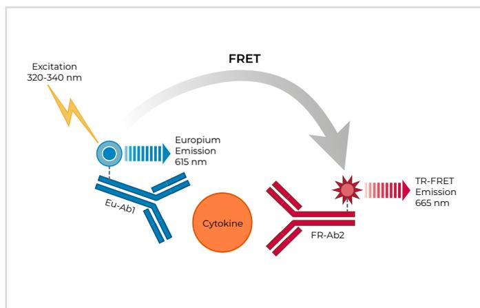
Figure 1 Schematic representation of the TR-FRET assay principle.
